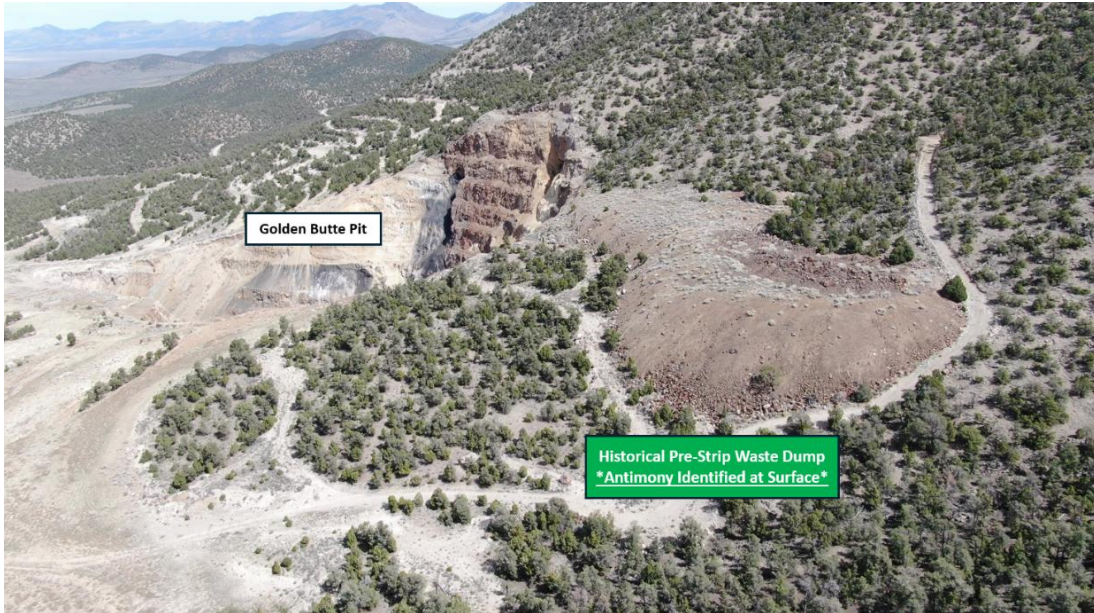
Figure 2 – Drone picture at Limo Butte looking northeast with newly defined antimony mineralization at surface in historical pre-strip waste dump adjacent to the historically mined Golden Butte pit. To view image please click here
