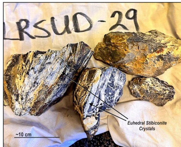
Figure 2 - Selective rock chip sample LRSUD-29 grading 16.27% Sb and 0.16 g/t Au , with coarse euhedral stibiconite, antimony oxide mineral, crystals embedded in a silicified matrix. To view image please click here
